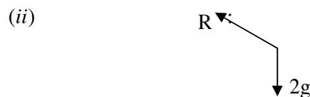
$$\begin{aligned} (iii) \quad R \sin 30 &= 2g \\ R \left(\frac{1}{2}\right) &= 20 \Rightarrow R = 40 \text{ N} \end{aligned}$$
